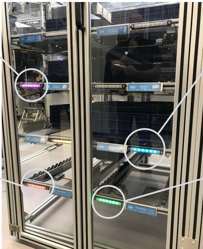
P2L shows the right lane and gives feedback to the workers
